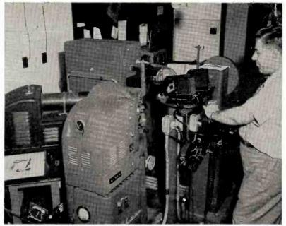
WBEN-TV utilizes a complex 6-way set-up with film camera. Two 2" x 2" slide projectors, two movie projectors, a Baloptican and a Kaleidoscope projector are utilized. Quentin P. Renner is station's film editor.
