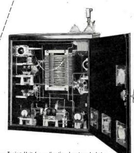
Special Antenna Tuning Unit for a directional system. Includes pattern switching and isolation coil for sampling cable.
