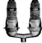
SINGLE and DOUBLE OBSTRUCTION LIGHTS Precision machined for proper light center. Heavy aluminum alloy castings. Prismatic globes meet CAA specifications. Drainage ports for condensation. Mounting base for standard A-21 signal lamps.
