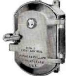
AUTOMATIC TOWER LIGHT CONTROL — "PEC" SERIES Specifically designed for radio tower use. Turns lights an at 35 f.c.; off at 58 f.c. as recommended by CAA.
